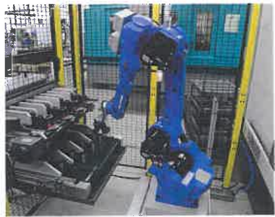
Figure 5.7: Simple and ingenious: the positioning of the robot on an inclined base next to the machine allows perfect accessibility to the machine (Photograph: Ralf Högel)
