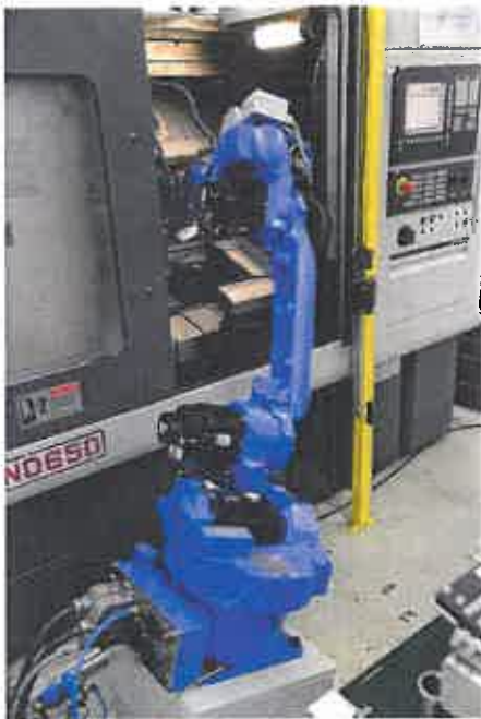
Figure 5.7: Simple and ingenious: the positioning of the robot on an inclined base next to the machine allows perfect accessibility to the machine (Photograph: Ralf Högel)
