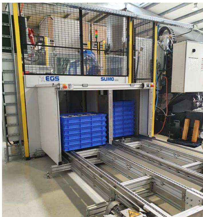
The second face of the workpieces is milled in a second machine, a Brother Speedio S700. Here again, automatic loading takes place laterally through a specially designed loading door. The machining of the second side is far less complex, significantly shorter and done individually.
