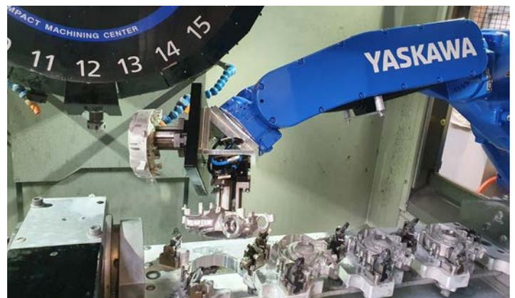
The starting point for the automation process was an existing Brother Speedio S1000 machining centre, in which one side of the workpieces is machined in four-part clamping. The aim was to convert the existing clamping fixture, into which the components were previously inserted manually, to automatic loading with as few modifications as possible.
